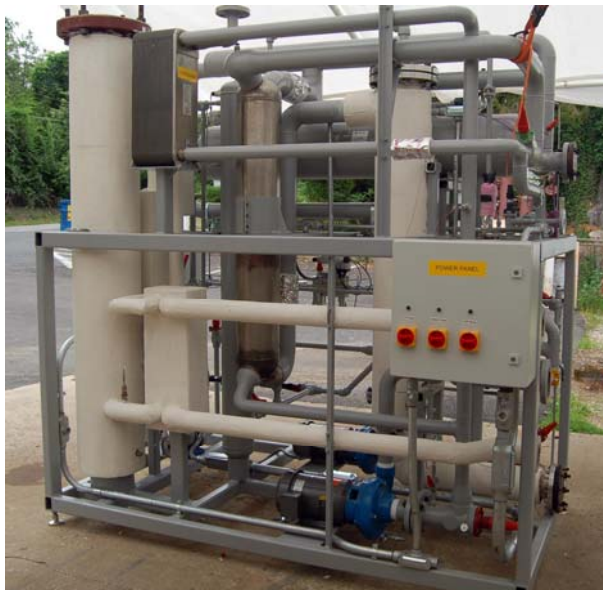
Pictured above is a field demonstration THP with 300 kW (one million BTU/hour) of useful heating plus 120 kW chilling (35 tons) from 180 kW (610,000 BTU/hour) heat input.
